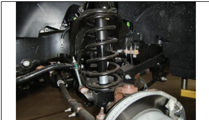
Picture of front suspension. Support front axle with jack.
