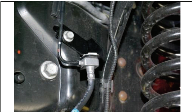
Reinstall block into bracket with retaining clip.
