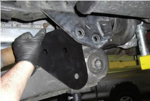
Carefully lower arm enough to slide drop bracket into frame.
