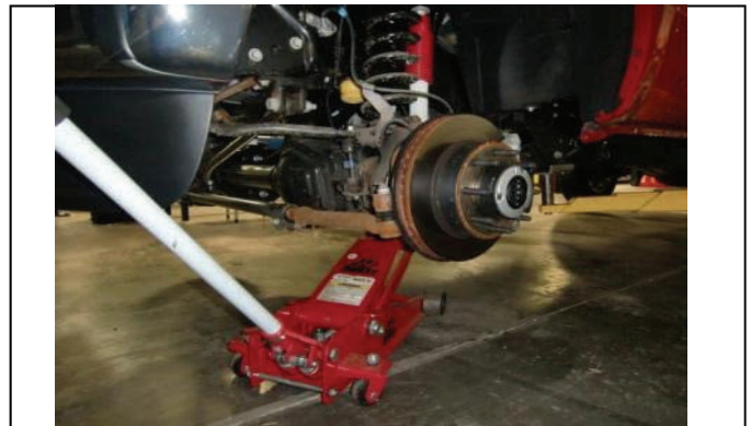
Support front axle with floor jack(s).
