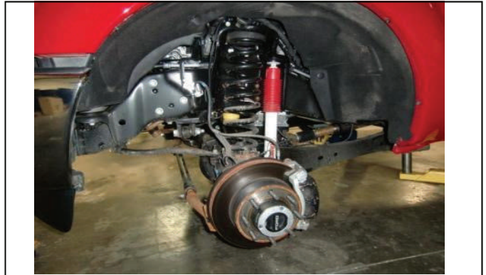
Remove front wheels and tires.
