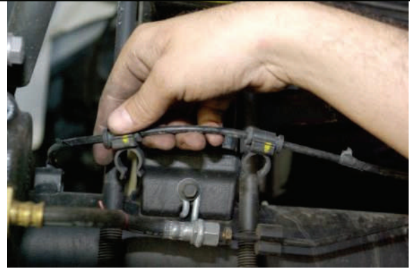
Vehicles with ABS/TC remove clips from U-bolts.
