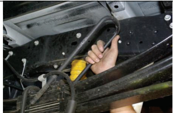
Remove U-bolts and slowly lower axle to remove OE block.
