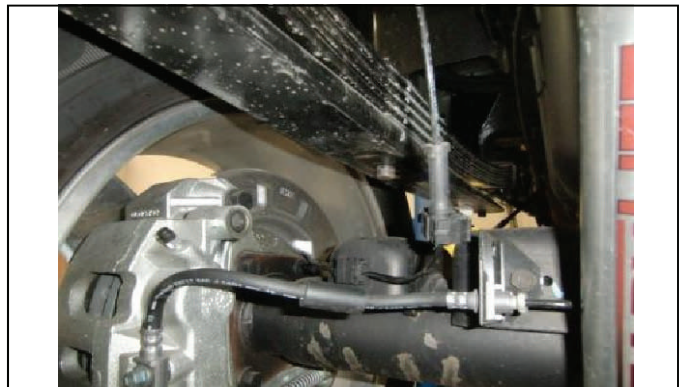
Carefully lower axle enough to install lift block
