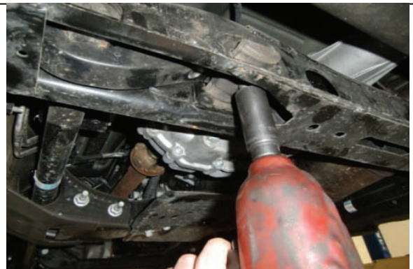
Adjust torsion bars to approx ride height
