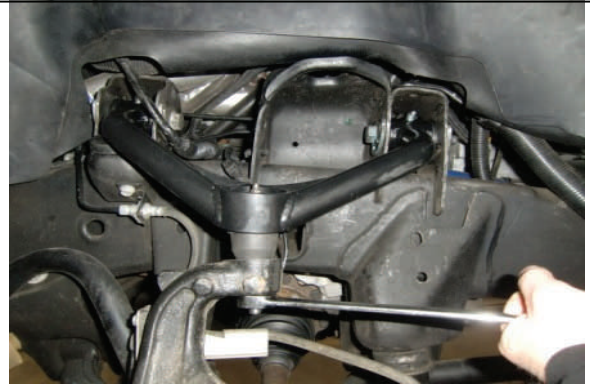
Connect upper ball joint to spindle
