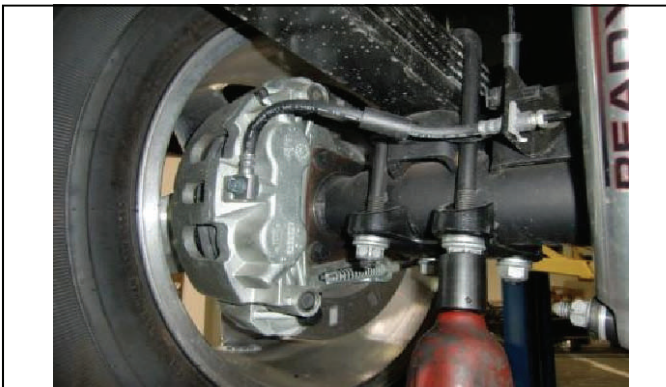
Loosen and remove u-bolt hardware
