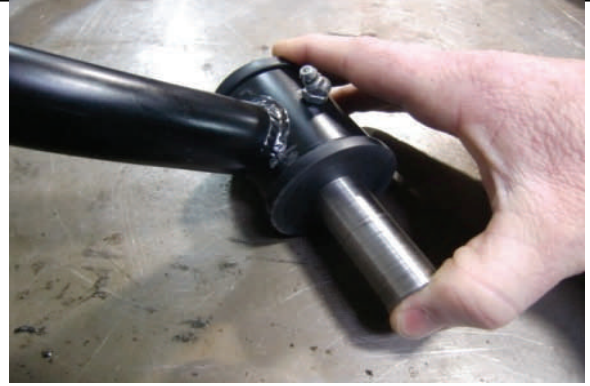
Assemble bushing halves and insert crush sleeves
