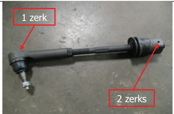
Locate new assembled HD steering kit and install zerk fittings
