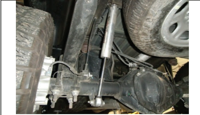
Longer shocks recommended for this kit use RL# 69-3411R
