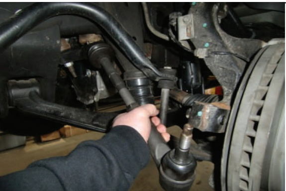
Install new steering assembly on center link
