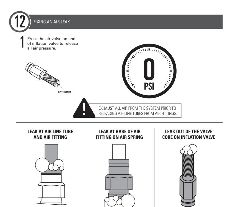
Release air line tube (see page 11). Review proper cuts and procedures in Step 8. Repeat Steps 9 and 11.
