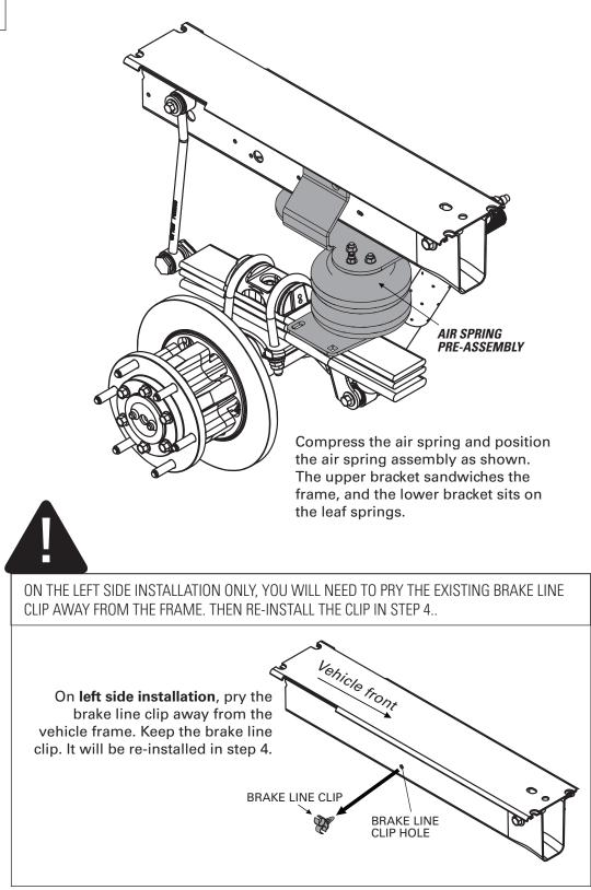
SECURE AIR SPRING PRE-ASSEMBLY TO VEHICLE FRAME
