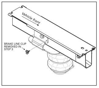
Re-install the jounce bumper cup with the jounce bumper cup bolt. Tighten to factory specfications.
