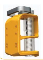
Steel spring is mounted inside the pin to protect it from impact damage. Keyway is designed into the pin, and the key is designed into the frame. This eliminates the need to 'hunt' for the keyway when opening and closing.
