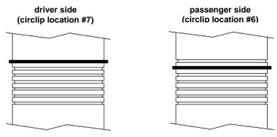
On 4x2 models, it is recommended that the driver side circlip is installed two positions higher than the passenger side circlip. For example, to achieve the only offered lift setting of 2.55", the circlips should be installed as follows (Note: Do not use circlip locations #4, #5, #6, or #7 on 4x2 models):
