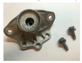
**C.** Install the new Bilstein B6 shock absorber on to the OEM top mount. Make sure to install the top mount in the same orientation it was removed from the vehicle.
