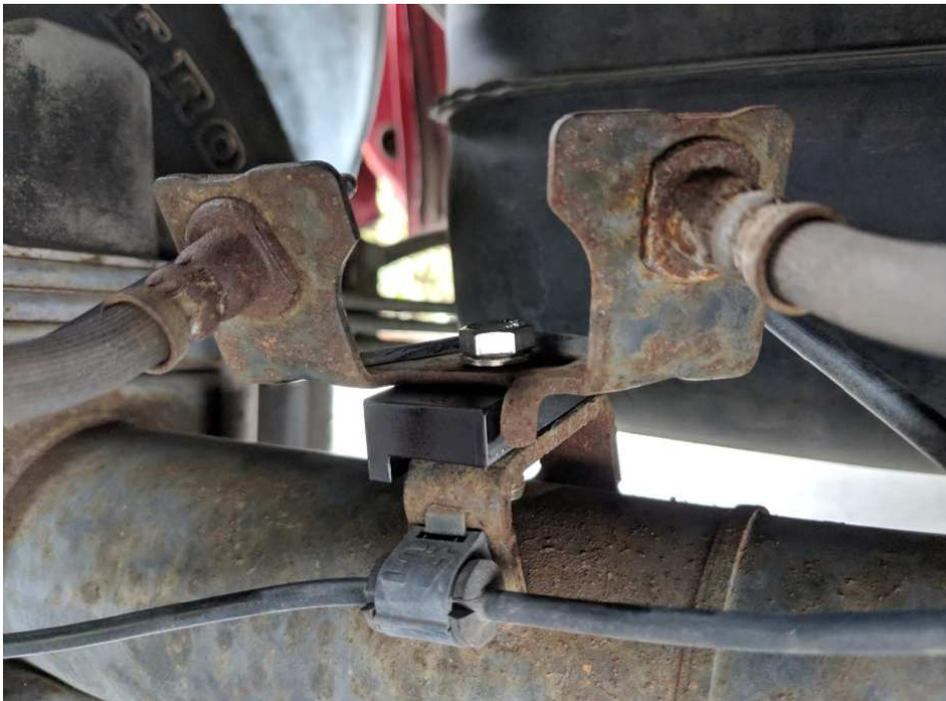
3. Install the lower end of the shock absorber with the bolt, nut and washer. Temporarily hand tighten.
