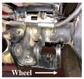
Figure 13 - Passenger Side Offset Bracket
