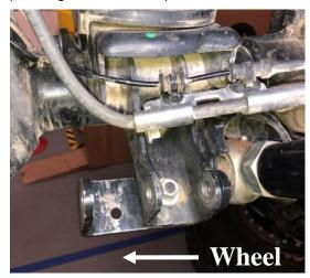
Figure 12 - Driver Side Offset Bracket
