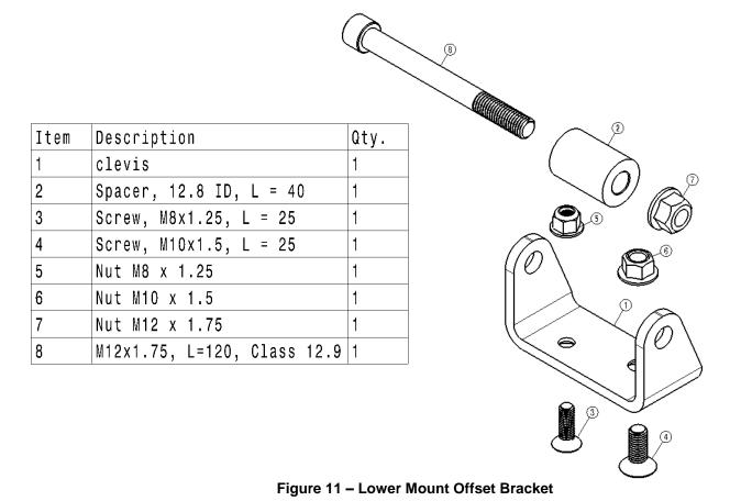
O. Install the clevis from the mount kit in Figure 11 as shown in Figures 12 & 13. The position of the clevis should allow the shock lower mount to be offset outboard towards the wheel. Use the M10 screw and nut for driver side and torque fastener to 31 lb•ft (42 N•m). Use M8 screw and nut for passenger side and torque fastener to 19 lb•ft (25 N•m).
