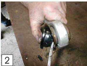
**NOTE:** Reuse OEM sleeves & **DO NOT REMOVE** metal shells, they are reused.
