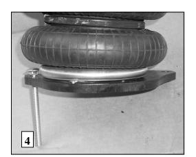
4. Insert a carriage bolt in the forward square hole and attach air spring to plate using the 3/8 x 1" flat head cap screw provided. Torque to 20-25 ft-lb.
