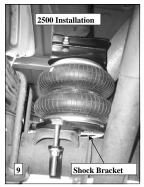
9. On 2500HD installations, it may be necessary to trim the corner of the shock bracket 1/16" - 1/8" to allow the plate to sit flush on axle pad.
