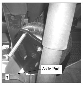
7. Compress air spring assembly and place on top of bump stop plates on top of the axle pad. MAKE SURE THAT THE ASSEMBLY WILL NOT DAMAGE OR CRUSH BRAKE LINES, WIRING HARNESSES, OR EMERGENCY BRAKE CABLES.
