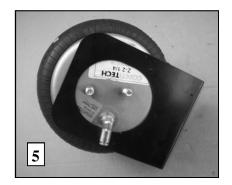
5. Place heat shield over top of air spring assembly as shown. (Passenger side shown. Drivers side heat shield is oriented to front of vehicle) Driver's side heat shield must be oriented to keep emergency brake cable from rubbing on air spring.
