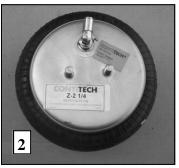
2. Install elbow fitting in port of air spring. Torque fitting to approximately 20 ft-lb. Make sure that fitting is oriented as shown in photo.
