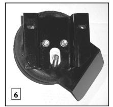
6. Place frame bracket over air spring assembly and attach using 3/8" flange nuts. Torque nuts to 20 ft-lb. Passenger side shown.
