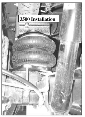
8. Slide spacer plate with two slotted holes between frame rail and upper bracket as shown in photos and attach assembly to frame rail using  $3/8 \times 1$ - 1/4 bolts and flange nuts. Check alignment of heat shield and torque nuts to 20-25 ft-lb.
