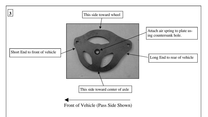
3. Lay out base plate as shown in photo. The air spring mounting hole is countersunk on both sides to allow the plate to be oriented correctly for both the left and right sides of the vehicle. (Passenger side shown) Attach air spring to plate using 3/8" flathead bolt. Tighten to 20 ft-lb.
