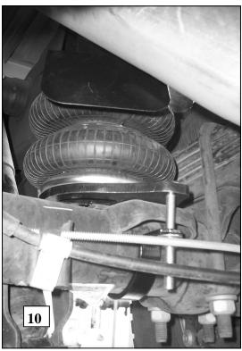
10. When the assembly is aligned properly, install axle strap using carriage bolts and remaining nuts and washers. It may be necessary to flex the brake lines slightly to allow clearance for the axle strap. MAKE SURE AXLE STRAP AND CARRIAGE BOLT WILL NOT CONTACT BRAKE LINE. Tighten nuts until the strap ends flex slightly. The carriage bolts are designed to be long enough for the 3500 HD installation. For 2500 HD applications they can be cut shorter if desired.
