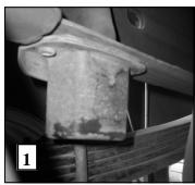
1. Park vehicle securely and set parking brake and chock wheels. Remove factory bump stops from vehicle by removing nuts from studs using a 15mm wrench or socket
