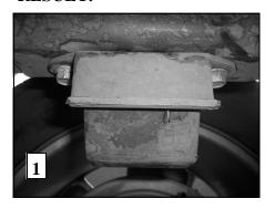
1. Park vehicle securely and set parking brake and chock wheels. Remove factory bump stops from vehicle by removing nuts from studs using a 15mm wrench or socket
