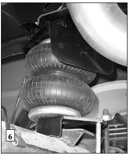
6. Insert assembly between frame rail and axle and attach frame bracket using supplied M10-1.5 x 30 flange bolts to existing threaded hole in frame. Align bracket and torque bolts to 20-25 ft-lb.
