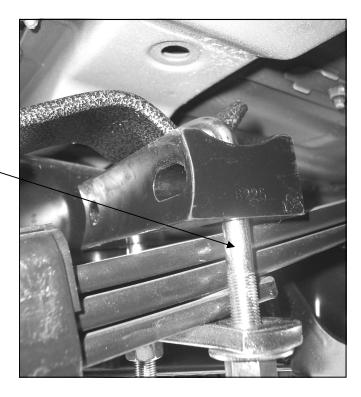
Install Long offset U-bolt as shown with 9/16" Hardware.
