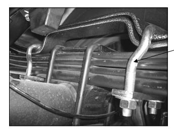
Install Short offset ubolts as shown using 9/16" hardware.
