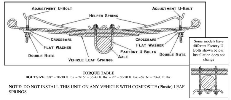
**NOTE**: IF THIS UNIT IS TO BE INSTALLED ON ANY DODGE VAN OR MOTORHOME CHASSIS MODEL NUMBERS, B300, B400, MB300, MB400, F30, F40, OR F44 WITH THE PLASTIC MOLDED GAS TANK, A SPECIAL CLEARANCE BRACKET IS REQUIRED AND IS AVAILABLE THROUGH YOUR LOCAL DEALER OR THROUGH HELLWIG PRODUCTS CO.
