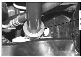
Install collar clamps inboard of frame bushings to keep sway bar centered.
