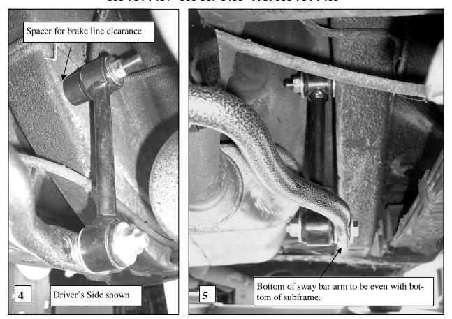
**TORQUE TABLE** Bolt Size 3/8"— 35 ft lbs \* Bolt Size 7/16"— 45 ft lbs \* Bolt Size 1/2"—75 ft lbs \*Bolt Size 9/16"— 90 ft lbs
