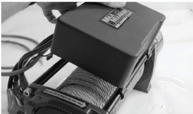
2-9: Mount Control Box on the Tie Bars.
