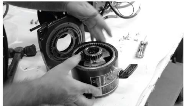
1-4: Separate Leg and Gear Housing.
