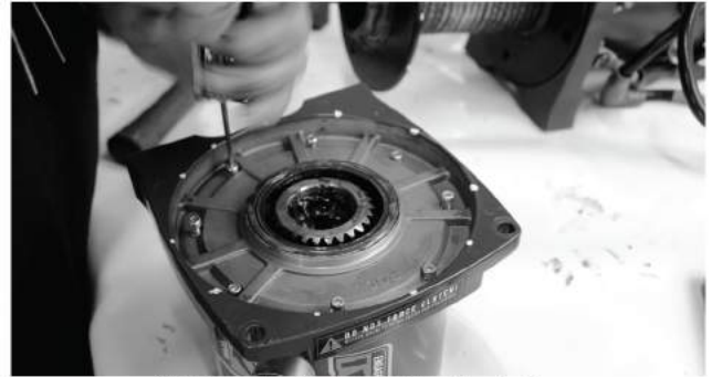
1-3: Remove the 8 bolts in the Gear Housing Leg.
