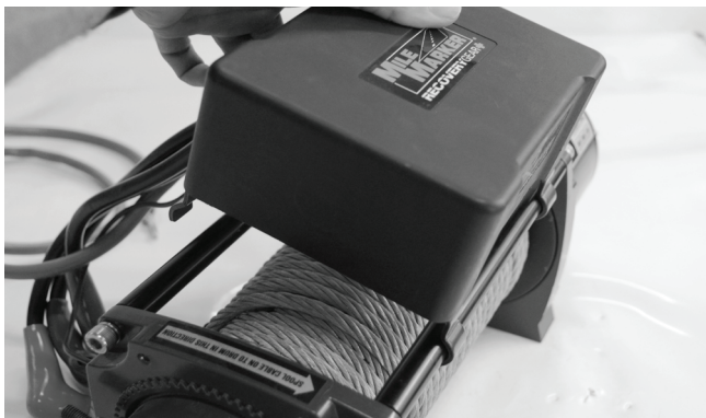
2-9: Mount Control Box on the Tie Bars.
