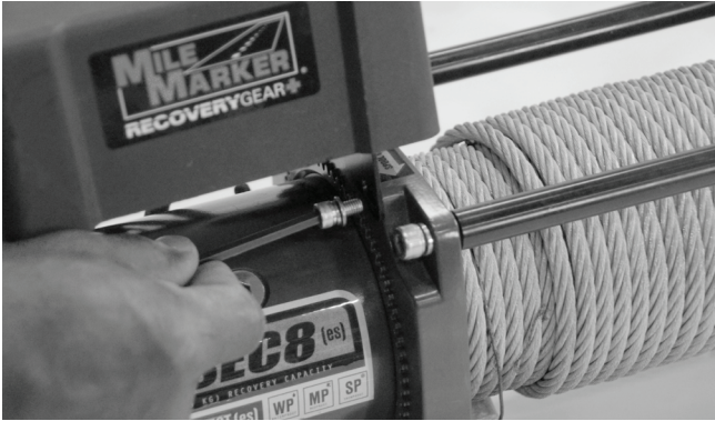
2-5: Screw bolts with control box in the mounting points.
