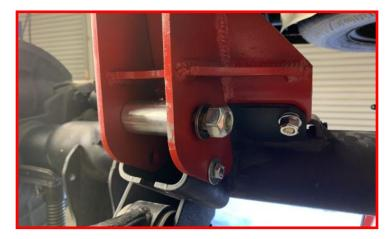
Install the upper control arm into the upper control arm bracket using the factory pivot hardware. Do not tighten at this time. With the upper control arm installed. Tighten all bracket mounting hardware in order.
