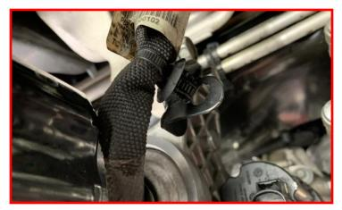
Remove the actuator harness retaining clip from the inside the frame rail.
