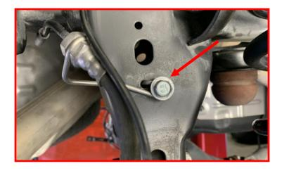
Remove the passenger ABS retaining clip at the frame rail.
