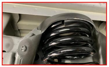
Note: Orientate the coil so the final coil terminates at 9 o'clock on the axle side.
