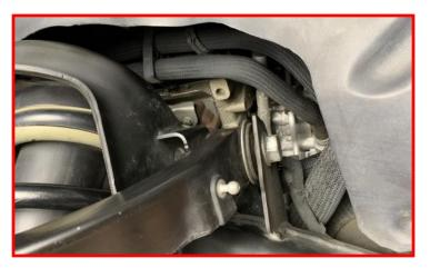
Loosen but do not remove the lower control arm ball joint nut. Strike the lower ball joint boss on knuckle with a dead blow hammer to dislodge the taper. Remove nut and then the knuckle from the vehicle.
