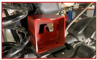
On the driver side only, Install the bump stop nut plate.
