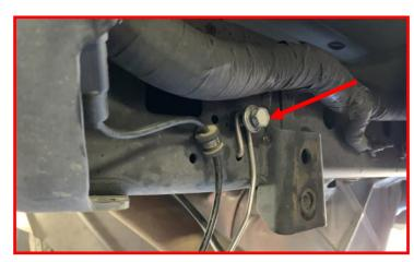
Remove the driver ABS retaining clip at the frame rail.
