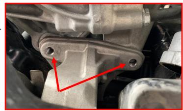
Remove (2) passenger side differential mounting bolts. Retain the factory hardware.
