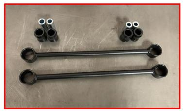
Install the urethane bushings and sleeves into the end links using the supplied grease pack. Use a light amount of grease on the bushing and press into the end link.
