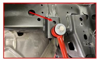
Install the completed sway bar end link assembly onto the sway bar using the supplied M12 x 70mm bolt, nut, flat washer and fender washer. Do not tighten at this time.
