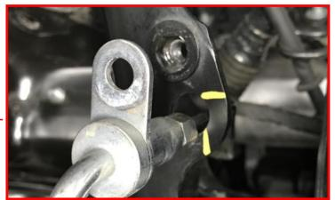
Remove brake line from factory mounting area.
