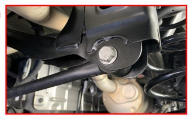
Lower the axle down enough to remove the springs and rubber isolator.
