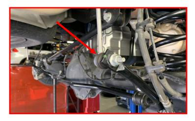
Locate and remove the passenger brake line bracket mounted on the frame rail.
