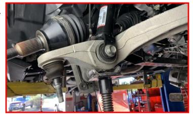
Loosen but do not remove the lower control arm pivot bolts.
