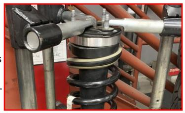
Locate the top strut extension and install using the factory hardware.
