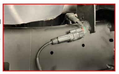
Route the ABS wire between the knuckle and the strut. Ensure the ABS wire is routed over the CV axle as well.
