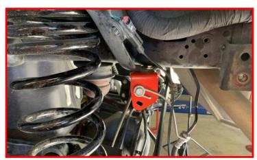
Install the ABS retaining clip into the driver rear brake line bracket in the bottom hole. Tighten the bracket at this time.
