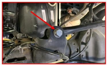
Loosen the frame side track bar mounting bolt.
