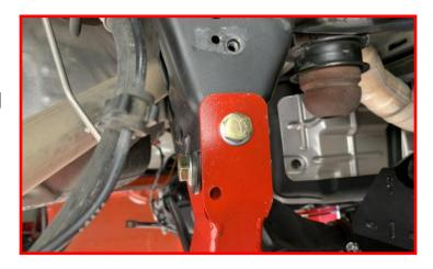
Note the location and orientation of track bar bracket nut plate.
