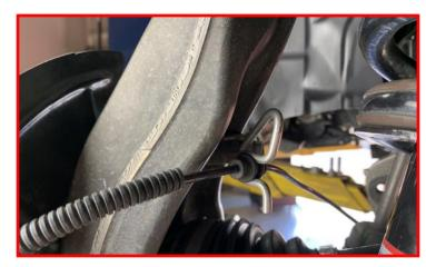
Loosen but do not remove the upper control arm ball joint nut. Strike the upper ball joint boss on knuckle with a dead blow hammer to dislodge the taper. Remove nut and let knuckle hang out of the way.
