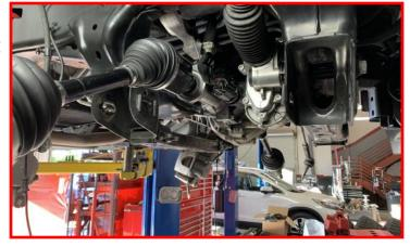
Remove the (4) rear crossmember mounting bolts. Remove crossmember from the vehicle. Discard the crossmember and mounting hardware.
