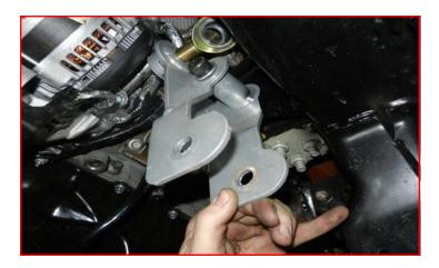
Install the ReadyLift passenger side differential drop into the factory location using factory hardware. Do not tighten at this time.
