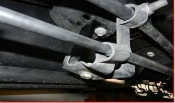
Install rear wheels and lower vehicle to the ground. Torque lug nuts to wheel manufacturers specifications. Jounce vehicle to settle suspension. Torque rear u-bolts to 110 ft-lbs, and shock hardware to 60 ft-lbs. Install the vehicles power source at the ground terminal.
