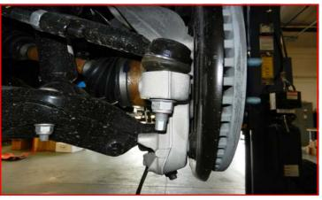
Remove the caliper from the knuckle and hang out of the way using suitable hook. DO NOT let the caliper hang by the brake hose. Remove the brake rotor and dust shield. Remove the axle nut dust cover. Remove the axle nut.
