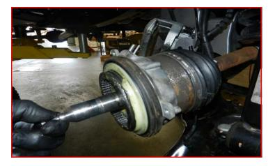
Install the ReadyLift knuckles onto the lower ball joints using factory ball joint nut, 3/4" washer. Run tight at this time. Will torque in later step.
