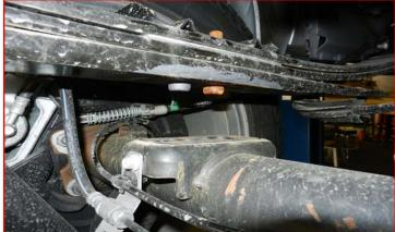
Locate the passenger side lift block, making sure the tapered end points to the front of the vehicle. Install the lift block on the axle pad aligning the pins. Raise the axle and the block up to the spring while aligning the center pins. Install the provided u-bolts, washers and nuts. Snug the u-bolt nuts but do not fully tighten at this time. Repeat steps for driver side.
