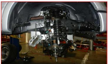
Remove hub assembly from the factory knuckles and transfer them to the Ready-Lift knuckles in the same orientation using factory hardware. Torque to 148 ft-lbs.
