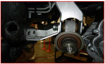
Install the ReadyLift sway bar brackets to corresponding sides of the frame using 7/16" x 1 1/4" bolts, flat washers, and lock nuts. Do not tighten at this time.
