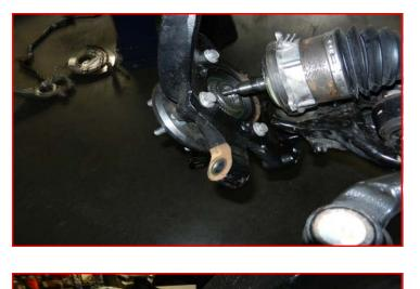
Take vacuum actuator and move to knuckle mounting surface making sure to engage the splined inner ring to the hub assembly and that the vacuum ports are pointing to the top of the knuckle. Install vacuum actuator using factory hardware. Torque to 132 in-lbs.
