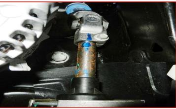
Disconnect the electrical leads to the rack and pinion. Support the rack and pinion and remove hardware from the frame. Carefully lower the rack & pinion assembly from the vehicle and set aside.
