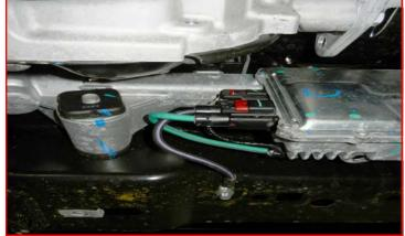
Measure from the outside edge of the driver side rear control arm pocket 2 5/8". Mark a vertical line on both the front and rear of the control arm pocket. Connect the 2 lines across the top of the pocket. Using a suitable cutting tool, cut this section off the frame. Sand and paint exposed metal with quality rust preventative paint.
