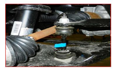
Remove the lower strut mount from the lower control arm.
