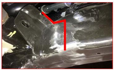
If your differential has the front assembly tab in the middle of the assembly, mark a straight line even with the housing and using a suitable cutting device, remove.
