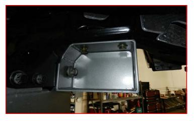
Install the ReadyLift rear cross member into the factory control arm frame pockets using M18 x 150mm bolts, flat washers, and lock nuts.
