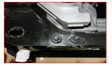
Mark driveshaft to differential location for installation later. Remove the driveshaft mounting bolts and allow driveshaft to hang out of the way.
