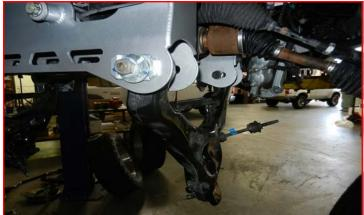
Tighten all differential, rack and pinion, and cross member hardware at this time. Starting with differential, torque all differential hardware to 95 ft-lbs, differential brace to cross member to 45 ft-lbs, cross member main hardware to 200 ft-lbs, sway bar drop bracket hardware to 60 ft-lbs, rack and pinion to front cross member hardware to 150 ft-lbs.
