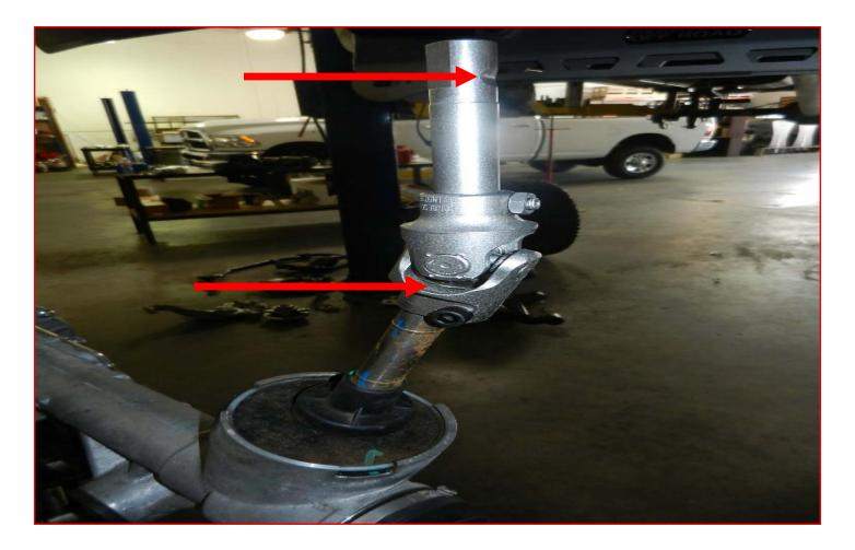
Locate the steering u-joint, and steering extension. Install the steering extension into the u-joint while making sure the pinch bolt on the u-joint and the pinch bolt slot on the extension are 100% in line with each other. Any position set other than this will cause the rack and pinion to steering wheel alignment to be off center and can cause failure of the clock spring inside the steering column.
