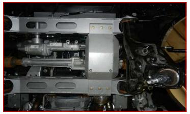
Install the ReadyLift driveshaft spacer and driveshaft in the same orientation with the marks previously made using the 10mm x 100mm Allen head bolts and a drop of thread locker to all bolts. Torque hardware to 50 ft-lbs.
