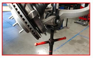
Remove the lower strut mounting hardware. Lower the control arm down while supporting the knuckle. Be mindful of the ABS and brake lines to not over extend them.
