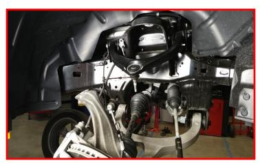
Remove the upper control arm from the frame.
