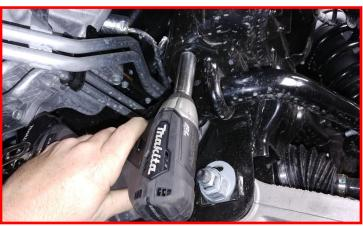
Install the front wheels and lower the vehicle to the ground. Torque the lug nuts to the wheel manufacturers specs.
