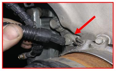
2019 and UP Models: Passenger side, locate the electrical harness on the coil over and follow it up onto the frame rail behind the plastic wheel liner.
