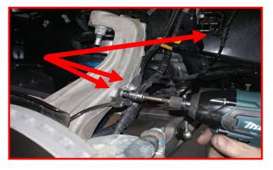
Remove the vacuum hose from the vacuum actuator on the knuckle.
