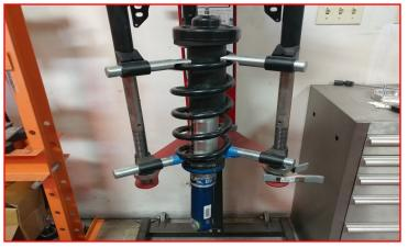
**1.5"** and **2.5"** kit top extension: Install the factory nuts onto the strut hat studs running them down until they bottom out. Using a suitable cutting tool, cut the studs off just above the nut. Remove the nuts and clean any off any burs. Paint the exposed metal with a quality rust preventative paint.
