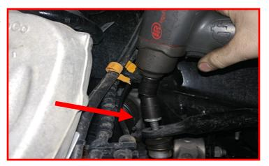
Remove the CV axle nut cover.
