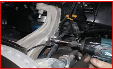
Install the sway bar end link onto the sway bar. Torque to 30 ft-lbs.
