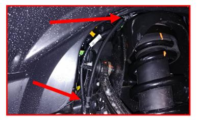
Mark another hole location in the plastic wheel liner in line with the original mounting hole but on the lower portion closest to the engine bay. Use a 7/16" drill bit and suitable drill to make the hole. Make sure to only drill through the plastic liner and not anything else. Move any wire harness that may be in the way to drill the hole. Install the coil over electrical connecter clip into the new hole.
