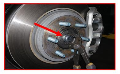
Remove the CV axle nut.
