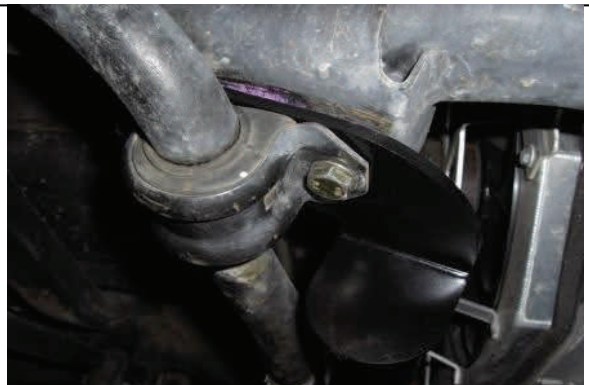
Start new hardware to reattach sway bar through bracket
