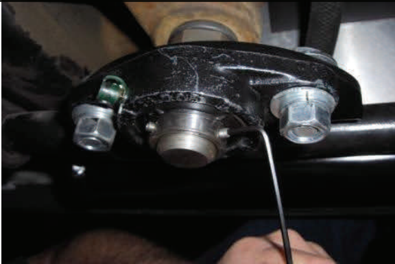
Attach bearing retainer and tighten set screws
