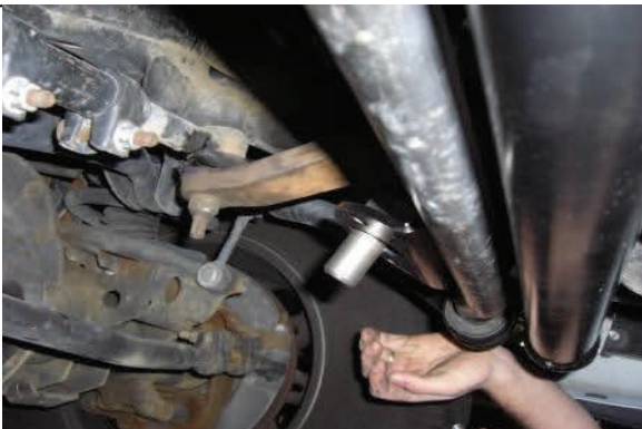
Place new stabilizer bar into position and raise sway bar
