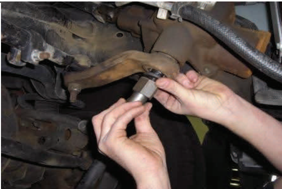
Place extension onto sector shaft with lock washer as shown
