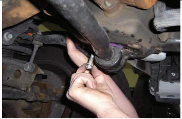
Remove sway bar mounting hardware at frame
