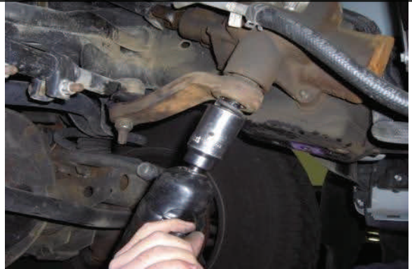
Remove pitman arm mounting nut
