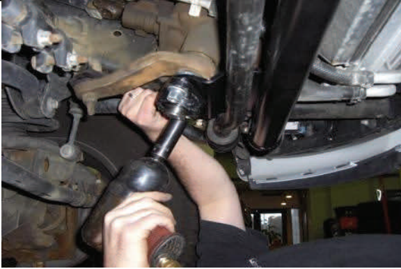
Attach locator bearing over sector shaft extension
