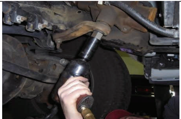
Tighten extension to factory specs
