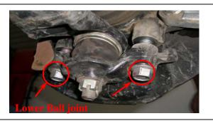
3. Loosen, don't remove the 19mm lower control arm nut and bolt, Remove the 19mm lower ball joint bolts.
