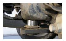
3. Install the 1" spacers between the differential supports and the front cross-member. Install the new bolts with factory washers and the new nuts and washers.
