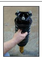
6. Reinstall the strut assembly in its stock location. Leave the three upper strut mounting nuts loose Raise the lower control arm and install the lower strut mounting bolt and nut. Use a floor jack to raise the lower control arm up in order to get the lower ball joint bolts installed. Be sure to use a thread locker on the lower ball joint bolts.
