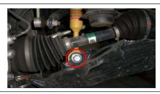
2. Starting from the passenger side, loosen the upper and lower strut mount nuts.
