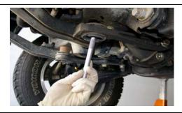
2. Remove the factory 19mm differential mounting nuts and bolts. The OEM washers will be reused.
