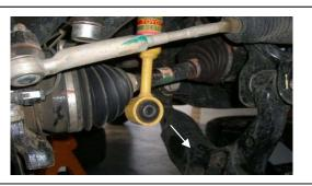
4. Remove the lower strut mount nut and bolt. Push the lower control arm down.
