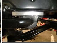
6. Sway bar spacer properly installed.
