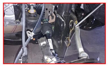
A helper is recommended for this step: Remove the 3 upper strut mounting nuts. Note the location of these nuts as 1 is different (outside most nut circled in red). This nut must be reinstalled in this location later. Remove the strut from the vehicle.
