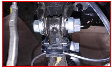
Install the ReadyLIFT sway bar bracket to the strut body using the provided M12 bolt, washers, and nuts. Install the sway bar end link to the bracket using the factory hardware. Torque all to 45 ft-lbs.
