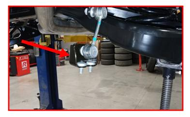
Install the ReadyLIFT sway bar bracket to the factory bracket using the provided M12 bolts, washers, and nuts and the end link to the bracket using the factory hardware. Torque all to 45 ft-lbs.
