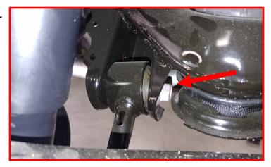
While supporting the lower control arm, remove the control arm to knuckle bolt.
