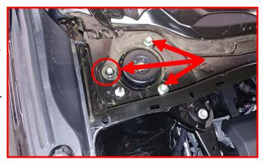
Install the ReadyLIFT strut extensions to the strut top hat using the provided M10 flange nuts. Torque to 30 ft-lbs.
