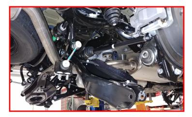
Install the ReadyLIFT spring spacer onto the spring keeping the factory isolator on top of the spring. Install the completed assembly into the subframe while raising the lower control arm into place.
