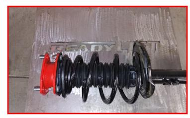
Install the completed strut assemblies back into the vehicle using the factory hardware. Only start the nuts by hand to allow movement when installing the knuckle. Make sure to install the hardware in the same locations as previously removed (outer nut circled in red).
