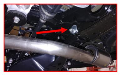
Loosen but do not remove the front lower control arm mount.
