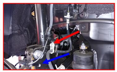
Locate the ABS wire bracket bolted to the inner fender well. Open the clamp that is holding the wire.
