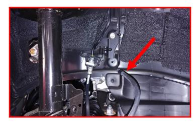
Remove the sway bar end link from the strut body. Let hang out of the way.
