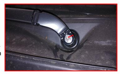
Locate the plastic rivets on both sides of the cowl plastic. There is one at both the driver and passenger sides on the outer edge closest to the engine bay. (Driver side shown)
