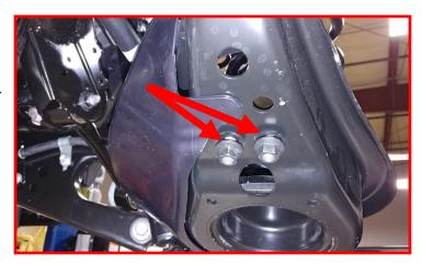
Loosen but do not remove the lower control arm cam bolt at the subframe.
