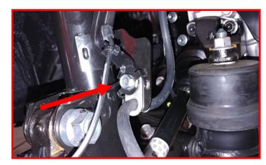
Install the ABS wire to the factory clip upside down from the direction it was previously. Pinch the clamp back to hold the ABS wire. Do not crush the wire.
