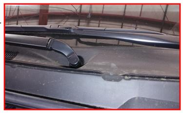
Mark the wiper arm and the shaft with a mark for reinstallation later. Remove the mounting nut. Remove the wiper arm by pushing gently down on the pivot point and pulling up on the mounting arm. These should pop off, though if your having a difficult time you can give the arm a little twist to help dislodge the taper. Set aside for reinstallation later.
