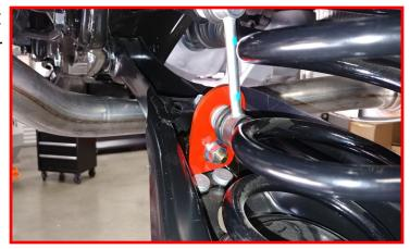
Attach the knuckle using the factory hardware. Torque to 110 ft-lbs.
