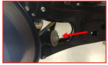
Loosen but do not remove the front lower control arm at the subframe.
