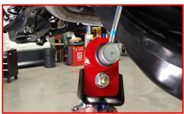
Install the completed end link and bracket assemblies to the lower control arm by rotating the sway bar up and end link into the bucket. Install using the factory hardware. Torque to 35 ft-lbs.
