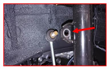
Remove the two bolts holding the strut to the knuckle.
