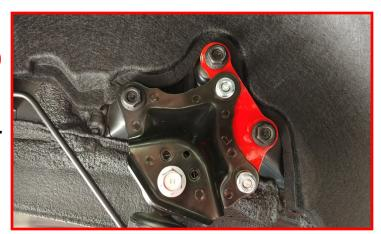
Using the jack, jack up the lower control arm on one side at a time to compress the suspension to ride height. This may take another jack at the opposite front corner under the subframe to stop weight transfer.
