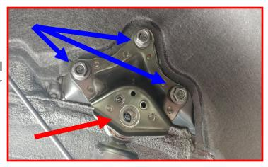
Remove the lower sway bar end link mounting bracket from the lower control arm. Rotate the sway bar up and then rotate the end link towards the back of the vehicle.
