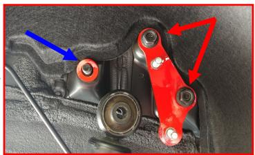
Install the factory shock mount to the ReadyLIFT mount using the provided M10 flange nuts and the back stud using the factory hardware. Torque the factory nuts to 45 ft-lbs, and the M10 nuts to 30 ft-lbs. Install the upper shock hardware. Do not tighten at this time.
