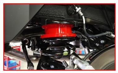
Remove the sway bar bracket from the end link.
