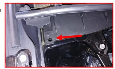
Once the rivets are removed, gently pull up on the leading edge closest to the engine bay. The clips holding the cowl plastic in place should release. Move the cowl out of the way.
