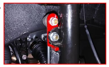
Install the brake line bracket and ABS bracket to the knuckle using the factory hardware. Torque to 5 ft-lbs.
