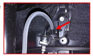
Remove the ABS wire from the bracket and let hang out of the way.
