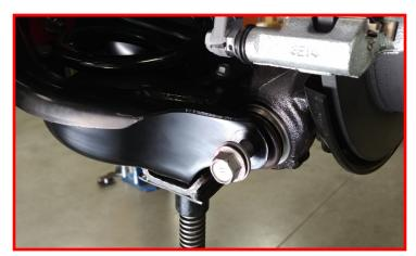
Lower the control arm down enough to remove the spring.
