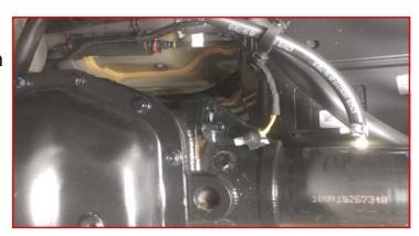
Remove the two harness clips from the frame cross member. You can clip these off the wire harness but is not necessary.
