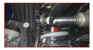
Remove the front lower shock from the axle.
