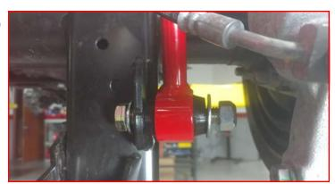
Install the ReadyLIFT rear shock extension using provided 1/2" x 1.25" bolt, washers, and nut. Use the factory bolt to line up the holes while tightening the 1/2" hardware. Once tight, remove the factory hardware.
