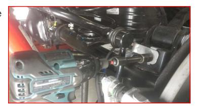
Remove the rear lower shock from the axle.
