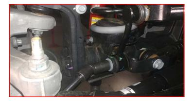
Remove the front sway bar end link from the sway bar. Discard as it will not be reused.
