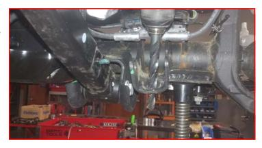
Install the ReadyLIFT front shock extension using provided 1/2" x 1.25" bolt, washers, and nut. Use the factory bolt to line up the holes while tightening the 1/2" hardware. Once tight, remove the factory hardware.
