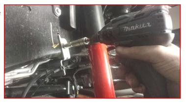
Remove the front brake line bracket at lower control arm.
