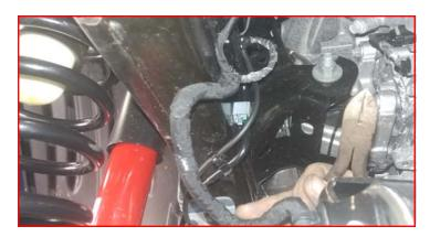
Locate the wire harness on the driver side frame rail and pull all clips out of the frame.
