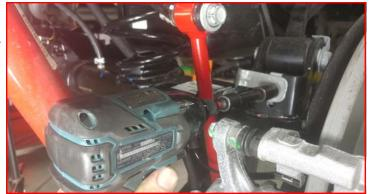
Install the ReadyLIFT brake line bracket to its corresponding side using the provided 1/4" x .75" bolt, washers and nut. Gently rotate/bend the metal brake line until you can line up the locking tab and bolt hole. Install using the factory hardware. Torque all to 5 ft-lbs.
