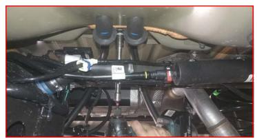
Remove the rear brake line bracket at the axle and frame rail.
