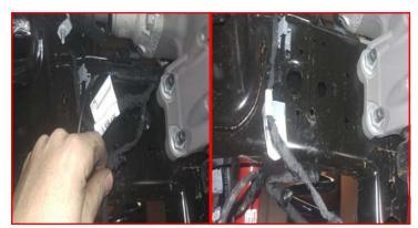
Using a suitable cutting device, clip the outside "Christmas tree" nipple off the electrical connector.
