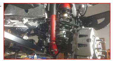
Install the factory rear end links to the sway bar and axle using the factory hardware. Torque to 45 ft-lbs.
