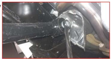
Loosen but do not remove the front upper control arms at the axle.
