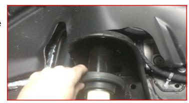
Install the ReadyLIFT front spacer, and then the factory isolator to the frame.
