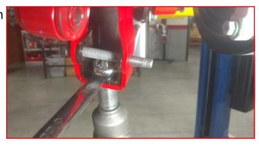
Install the ReadyLIFT crush sleeve and the factory hardware in the lower hole. Do not tighten at this time. Install the lower shock using the provided 1/2" x 2.75" bolt, washers and nut. Do not fully tighten at this time.
