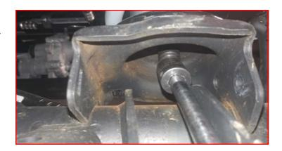
Locate the lower shock mounts on the axle and using a 1/2" drill bit, drill out the hole in the bottom of the mount.
