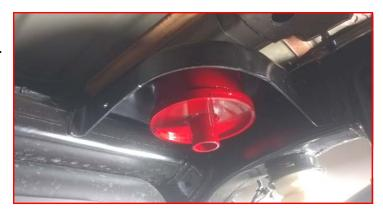
Locate the nipple on the coil spring isolator.
