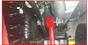
Install the ReadyLIFT sway bar end link to the axle using the provided 1/2" x 2.75" bolt, fender washer, flat washer and nut. Make sure to have the fender washer to the outside of the end link. Do not tighten at this time.
