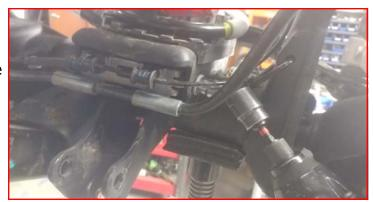
Install the provided 3/8" serrated flange nut to the 3/8" Allen bolt from the under side of the spring perch. Torque to 35 ft-lbs.
