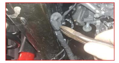
Cut the zip tie holding the "service loop" allowing the harness to extend.
