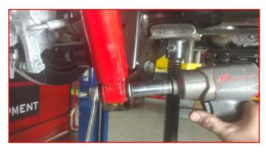
Remove the rear lower sway bar end link from the axle.
