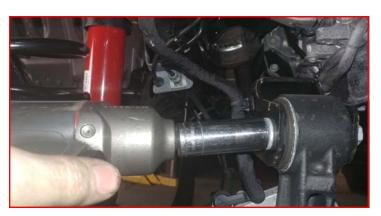
Mark the front drive shaft to pinion flange for reinstallation later.
