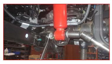
Loosen but do not remove the front lower control arms at the axle and frame.
