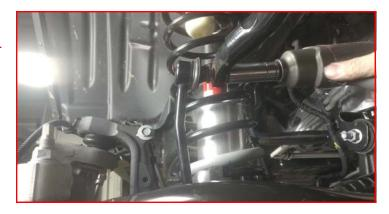
Install the electrical connector that was previously cut to the lower hole in the frame rail. The rest of the harness will hang.
