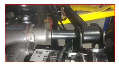
Loosen but do not remove the rear lower control arms at the axle and frame.
