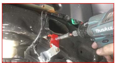
Install the ReadyLIFT rear bump stops to the axle using the provided 1/4" x .75" bolts, washers, and nuts. Torque to 5 ft-lbs.
