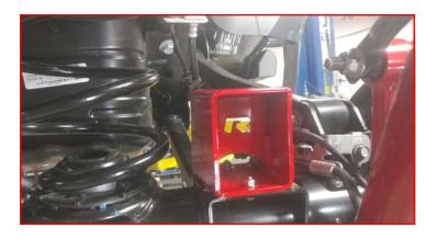
Install the ReadyLIFT e-brake cable to the body using the factory hardware and the factory e-brake bracket to the ReadyLIFT bracket using the provided 1/4" x .75" bolt, washers, and nut. Torque all to 5 ft-lbs.
