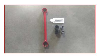
Install the urethane bushings and sleeves into the end links using the supplied grease pack. Use a light amount of grease on the bushing and press into the end link. Use a fair amount of grease on the inside of the bushing and press the sleeve into the bushing.
