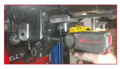
Loosen but do not remove the rear track bar at the axle and frame.
