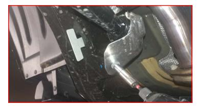
Gently bend the heat shield out of the way and loosen but do not remove the front upper control arm bolts.
