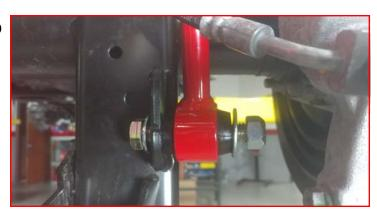
Install the ReadyLIFT rear shock extension using provided 1/2" x 1.25" bolt, washers, and nut. Use the factory bolt to line up the holes while tightening the 1/2" hardware. Once tight, remove the factory hardware.
