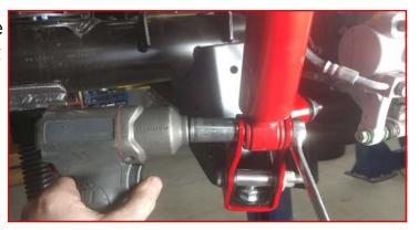
Install the brake line bracket to the axle using the factory hardware. Torque to 5 ft-lbs.
