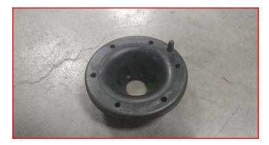
Remove the nipple off the rubber isolators using a suitable cutting device.
