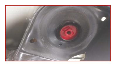
Install the ReadyLIFT rear spring spacer using the provided 1/2" x 2.25" Allen bolt. Torque to 25 ft-lbs.
