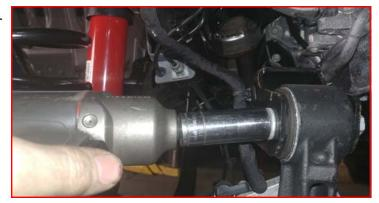
Mark the drive shaft to pinion flange for reinstallation later.
