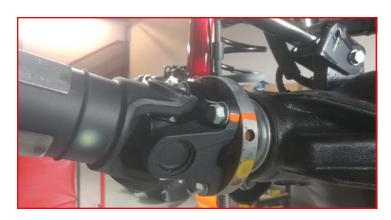
Remove the drive shaft from differential.
