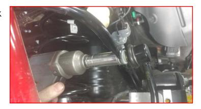
Loosen but do not remove the rear upper control arms at the axle and frame.
