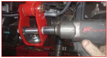
Install the brake line brackets to the lower control arm and frame rail using the factory hardware. Torque to 5 ft-lbs.
