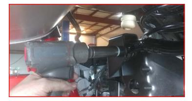
Lower the axle far enough to remove the springs. Make sure to note the springs orientation in the vehicle. They are top and bottom specific. Install the ReadyLIFT nut plate on top of the coil spring bucket.
