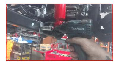
Remove the front sway bar end links from the axle. Save the hardware.
