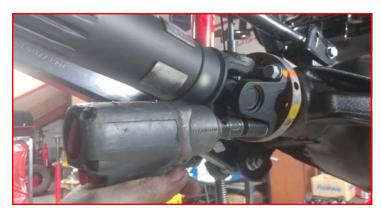
Lower the axle enough to remove the springs. Make sure to not over extend the brake lines or any other electrical harnesses. Remove the spring isolator. Using a suitable cutting device, remove the nipples just the same as the rear.
