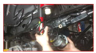
Remove the brake line bracket on the axle for access to install the bump stop nut on the passenger side.
