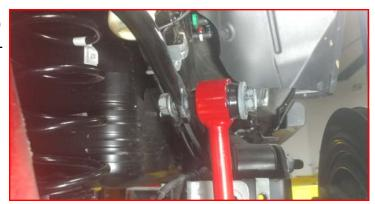
Install the ReadyLIFT sway bar end link to the axle using the provided 1/2" x 2.75" bolt, fender washer, flat washer and nut. Make sure to have the fender washer to the outside of the end link. Do not tighten at this time.
