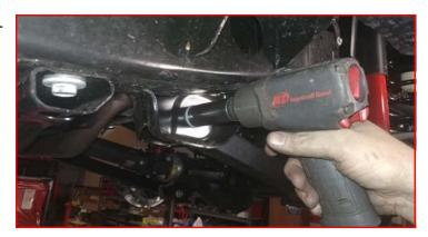
Remove the lower heat shield bolt from the front upper control arm pocket at the frame.
