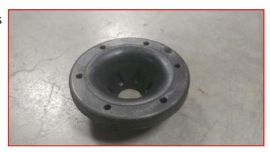
Install the spring and rubber isolator in the same orientation as removed. The springs are top and bottom specific. Raise the axle up enough to hold the spring assembly in place.
