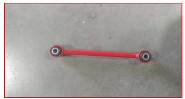
Install the ReadyLIFT sway bar end link to the sway bar using the factory lower hardware. Make sure to have the washer to the outside of the end link. Do not tighten at this time.
