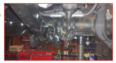
Install the ReadyLIFT front shock extension using provided 1/2" x 1.25" bolt, washers, and nut. Use the factory bolt to line up the holes while tightening the 1/2" hardware. Once tight, remove the factory hardware.
