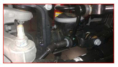
Remove the front sway bar end link from the sway bar. Discard as it will not be reused.
