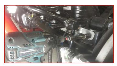
Remove the rear lower shock from the axle.
