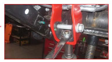
Install the ReadyLIFT crush sleeve and the factory shock bolt in the lower hole. Do not tighten at this time. Install the lower shock using the provided 1/2" x 2.75" bolt, washers and nut. Do not fully tighten at this time.
