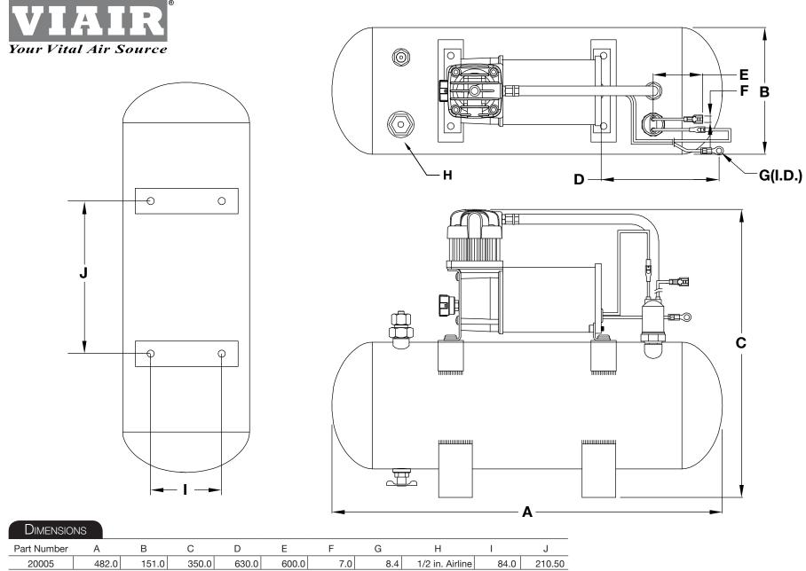
\* All measurements in millimeters, unless otherwise noted. \*\* All fittings are NPT, unless otherwise noted.
