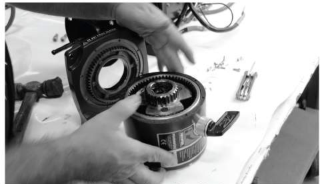
1-4: Separate Leg and Gear Housing.
